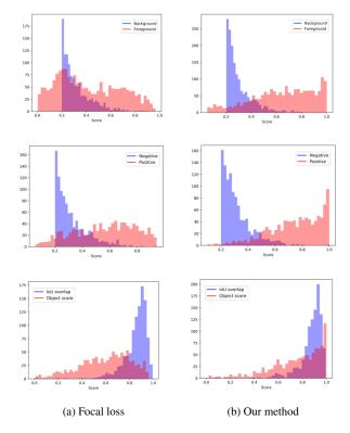
Figure 3. Comparisons of sample distribution. We plot foreground and background distribution (first row), positive and negative distribution for the person class (second row) and distribution of IoU overlap and object confidence score for the person class (third row). We select background / negative samples with score > 0.2for better visualization.
