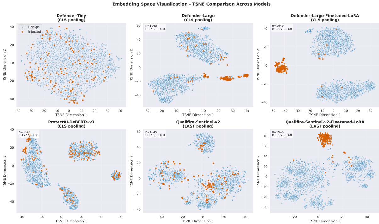
Figure 4: Visualizing the Domain Gap. t-SNE comparison of embedding spaces across model capacities of the real-world holdout set. Blue: Benign, Orange: Injected. While larger generic models like Defender-Large (top center) exhibit improved clustering consistent with their higher AUC, they still suffer from some overlap. In contrast, our Sentinel-v2 fine-tuned (bottom right) achieves near-perfect class separation, demonstrating that domain-specific adaptation is required to fully disentangle nuanced resume attacks.
