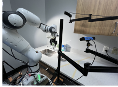
Figure 3: [LEFT] Our Franka DROID setup, annotated. [RIGHT] Franka DROID, including the top camera and right camera, moved to a new scene (kitchen sink).
