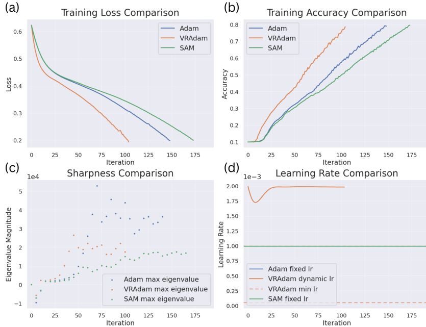
Figure 2: (a) Training loss curves for VRAdam, Adam, and SAM (Foret et al., 2021) of ResNet-32 on CIFAR-10 (b) training accuracy curves (c) plot of maximal eigenvalues of the loss Hessian (d) effective learning rate during training. Hyperparameters for these plots are provided in Appendix E.4.
