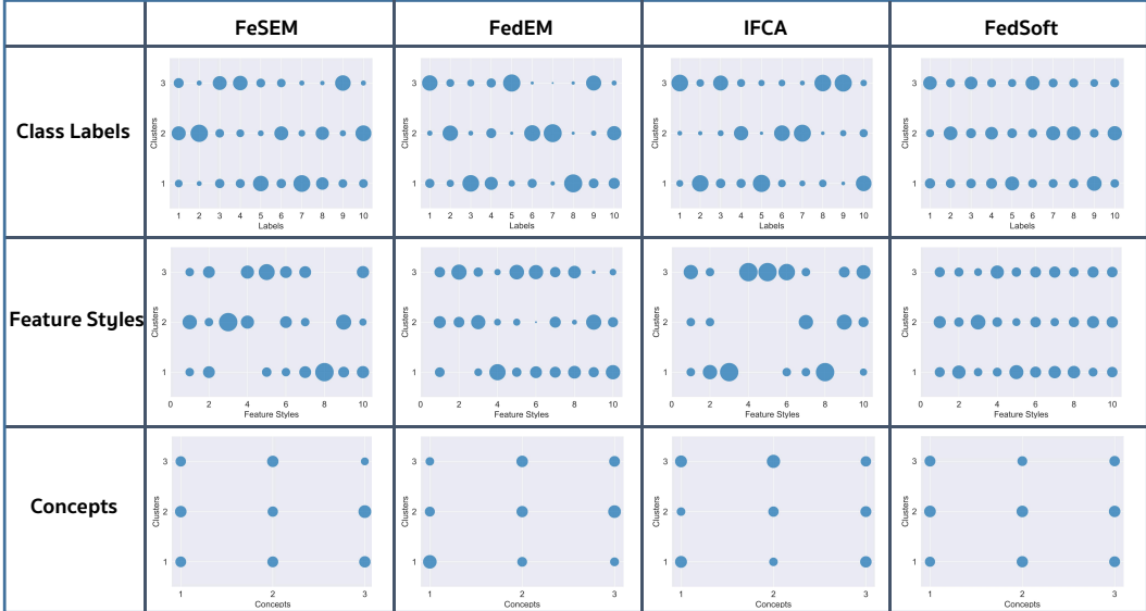
Figure 3: Clustering results w.r.t. classes/feature styles/concepts. After data construction, each data point x will have a class y , feature style f , and concept c . We report the percentage of data points associated with a class, feature style, or concept assigned to cluster k . For example, for a circle centered at position (y, k) , a larger circle size signifies that more data points with class y are assigned to cluster k . For feature styles, we only represent f \in [1, 10] here for clearer representation, and the full version can be found in Figure 12 of Appendix I. By the principles of robust clustering , we require a clustering method in which clients with the same concept are assigned to the same cluster (for example, Figure 4(b)).
