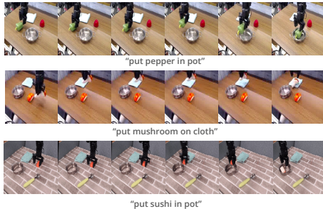
Figure 4: (Qualitative visualizations) V-GPS improves the precision of grasping the slippery object (first row), prevents the policy’s default behavior of releasing the object too early (second row) and holding the object for too long (third row). More qualitative results and videos can be found at https://nakamotoo.github.io/V-GPS
