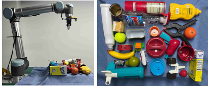
Figure 7: The robot setup of real-world experiments and the objects used for grasping.
