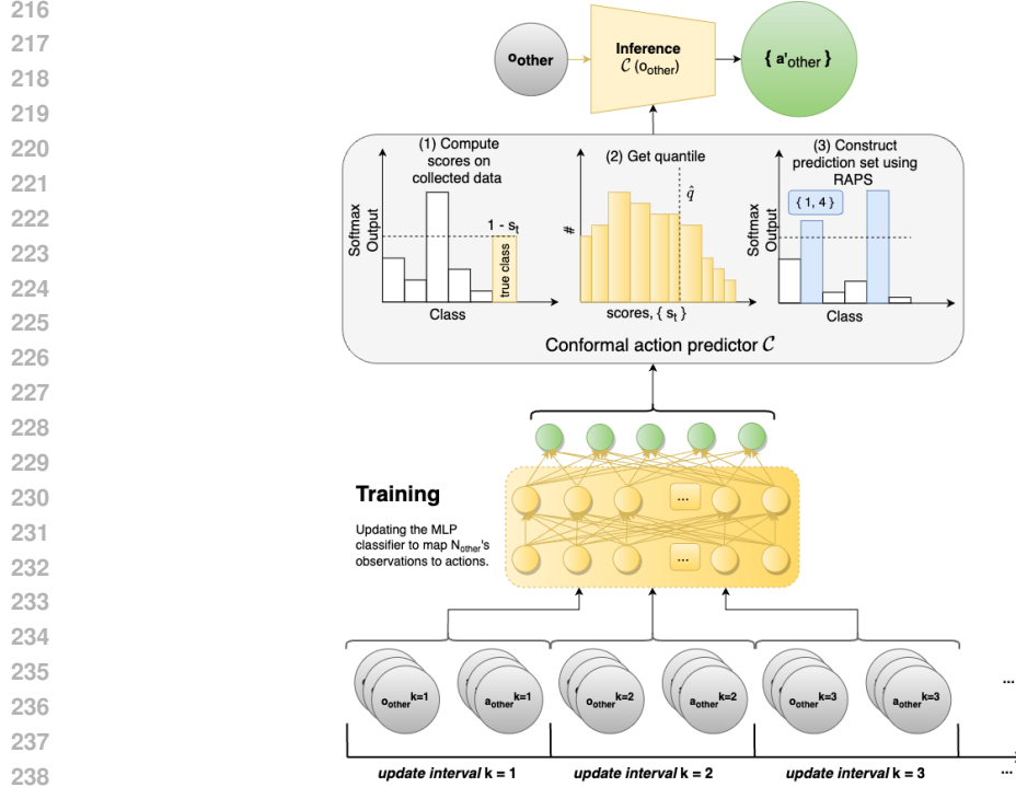
Figure 2: A detailed illustration of conformal action modelling and inference in CAMMARL to generate prediction sets of \mathcal{N}_{other} 's actions scores using conformal predictors.
