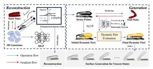
Figure 2: The overall pipeline of REArtGS. We introduce additional geometric and motion constraints for 3D Gaussian primitives, achieving high-quality surface mesh reconstruction and time-continuous generation, with only multi-view images from arbitrary two states.
