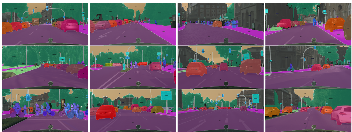
Figure 7: Qualitative results of panoptic segmentation generated by SimPLR on Cityscapes val. It can be seen that SimPLR correctly predicts small objects like pedestrians in various scenes.
