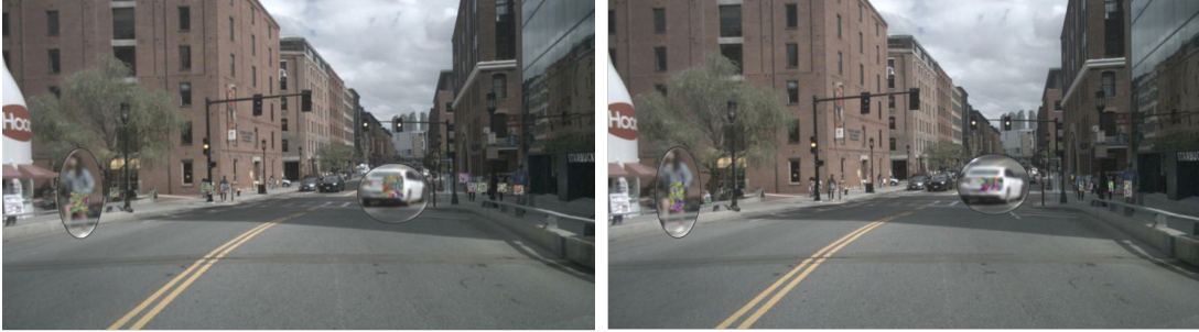
Figure 2: Illustration of adversarial patch size adaptations, wherein the patch size is adjusted proportionally to the target’s 2D bounding box dimensions. The left panel depicts a fixed-size patch, while the right panel presents a dynamically scaled patch.
