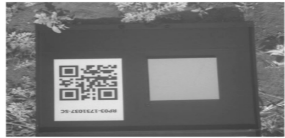
Figure 1: Calibrated reflectance panel which was used for data multispectral data acquisition.
