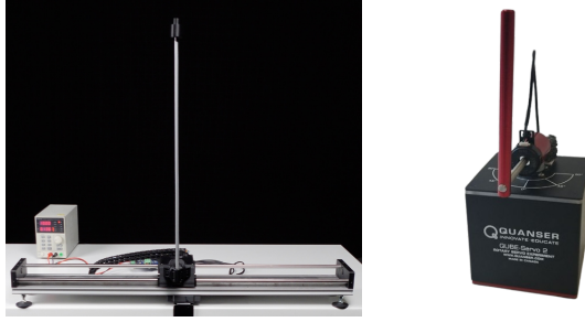
Figure 4: Custom cart-pole system on the left (image taken from (Anonymous, 2024)) and Quanser Qube Servo 2 Furuta systems on the right.
