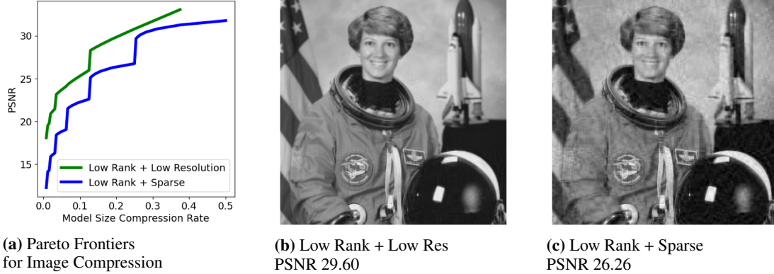
Figure 3: For a natural image, approximation as a sum of low rank and low resolution components (green points and subfigure b) achieves higher fidelity compared to the classic matrix decomposition as a sum of low rank and sparse components (blue points and subfigure c), with the same parameter budget (18.75% of the original image size, for subfigures b and c). The GA-Planes model family generalizes the idea of a low rank plus low resolution approximation to three dimensions.
