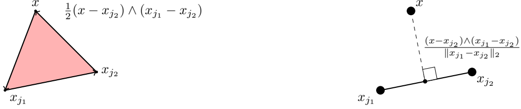
(a) The area of triangle formed by the points x , x_{j_1} and x_{j_2} is given by a wedge product.
