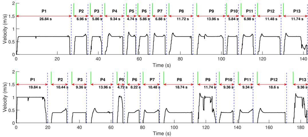
Figure 4: Velocity profiles and times for each navigation phase in the patrolling scenario. Top: *cohan*, Bottom: *cohan+platinum*.
