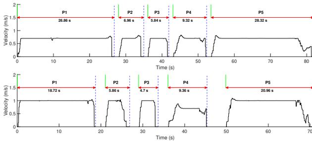
Figure 6: Velocity profiles and times for each navigation phase in the emergency scenario. Top: *cohan*, Bottom: *cohan+platinum*
