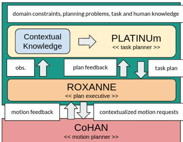
Figure 1: Integrated Task and Motion planning architecture.
