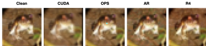
Figure 2: Comparison of the same image from different unlearnable datasets. OPS [19] perturbs by adding noise to a singular pixel. AR [16] generates perturbations using a sliding window approach. R4 [15] is a grid-like additive perturbation. CUDA and OPS, being unbounded methods, exhibit a noticeable perturbation, compared to AR and R4 which have perturbations bounded by an \ell_p -norm.
