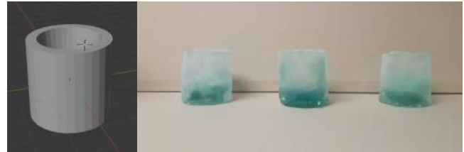
Figure 9: Left: the 3D model of the drinking cup. Right: three physical cups cast in ice.
