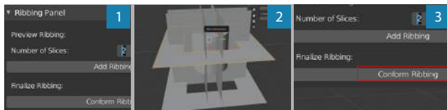
Figure 7: Creating ribbing with the FoldMold Pattern Builder. (1) Set number of slices to add along each axis. (2) Add ribbing to object and optionally transform slices around object for maximal support. (3) Select “Conform Ribbing” to finalize the ribbing shape.
