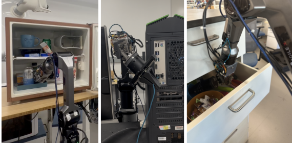
Fig. 6: The three tasks shown to evaluate the performance of the wrist as compared to the stock AgileX arm.
