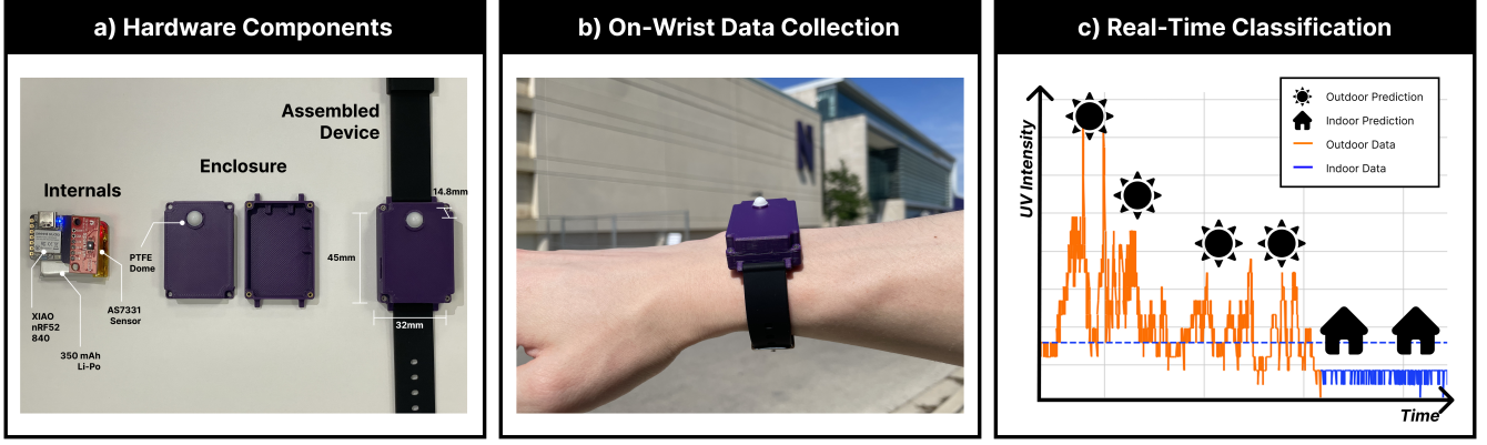
Fig. 1. System overview. (a) Hardware components: electronics assembly, enclosure with hemispherical PTFE dome, and fully assembled wearable. (b) Device worn on the wrist. (c) Example time series of UV measurements with corresponding logistic-regression output classification of indoor and outdoor segments.
