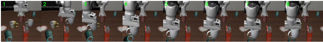
Layout - additional distractor objects lead to mislocalization of the target plate, with a nearby object being mistakenly recognized as the plate.
