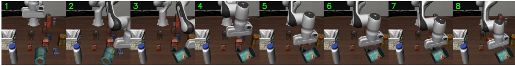
object - The model fails to flexibly rotate the robotic arm, resulting in a collision with a distractor object.
