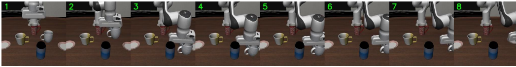
object - additional distractor objects lead to mislocalization of the target plate, with a nearby object being mistakenly recognized as the plate.
