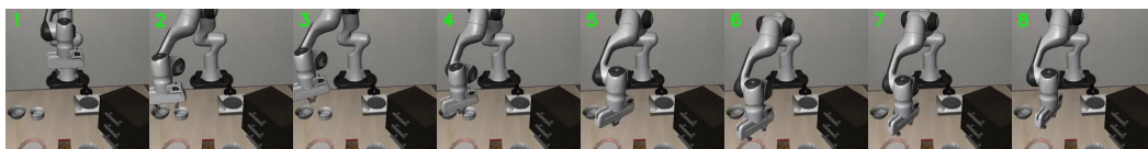
camera - changes in camera position cause the model to localize the target object inaccurately.
