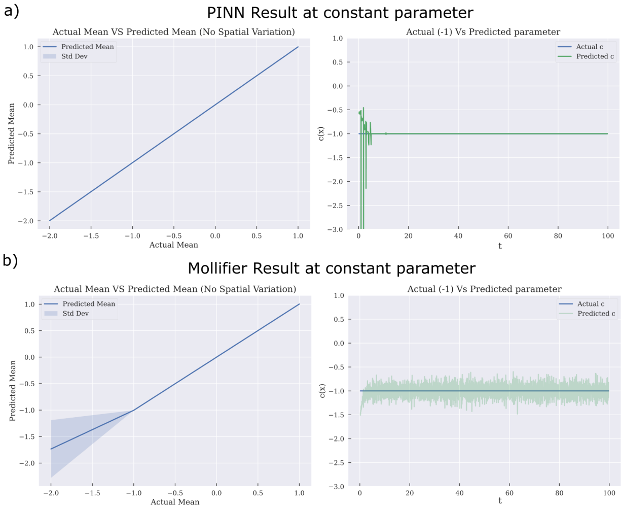
Figure 5: Constant forcing term inference in Langevin equation using PINN and Mollified PINN
