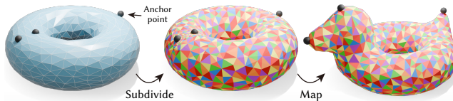
Figure 25: Our method allows base meshes with different shapes but with the same topology.
