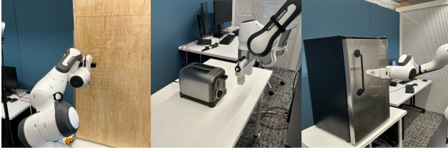
Figure 4. Real world environment setup. From left to right: push open door, push toaster lever, and pull open fridge door.
