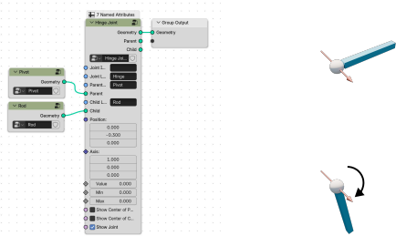
Figure 5. Simple Revolute Joint: Demonstrates a rod rotating about a pivot point using our custom hinge joint node.
