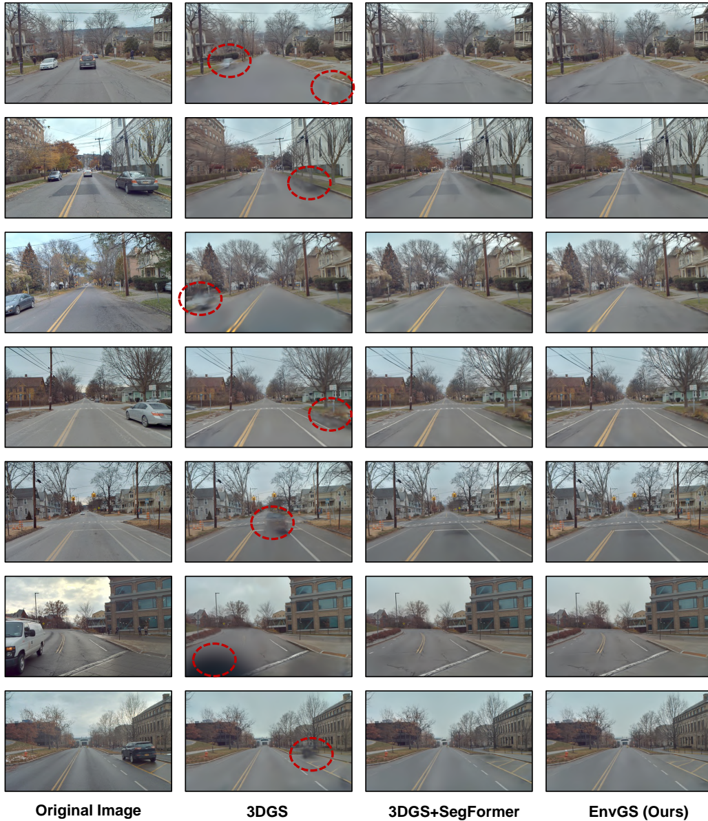
Figure XIV: Qualitative evaluations of the environment rendering. Our method demonstrates robust performance against transient objects.
