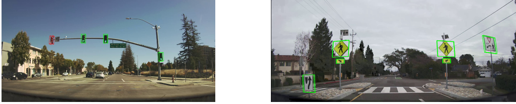
Figure 5: Samples from the dataset with 3D traffic sign and light annotations. The bounding boxes are automatically generated by our method. Traffic light states are color-coded.
