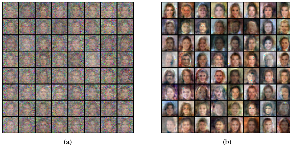
Figure 8: Model capacity vs. OOD detection. Images are generated from RealNVP trained on CelebA. Assume CIFAR-10 as OOD, and our GOD1KS and GOD2KS results are segmented by \perp . (a) Generated images from a RealNVP with 1 block and 2048 hidden channels. AUROCs = 0.98|0.99. (b) Generated images from a RealNVP with 16 blocks and 512 hidden channels. AUROCs = 0.88|0.88.
