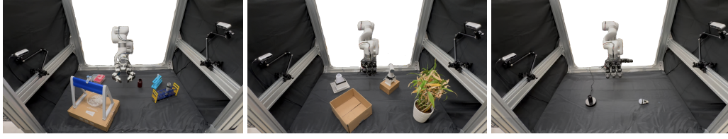
Figure 11: Environment Setup for the three dexterous manipulation tasks. Left: Liquid Handling. Middle: Plant Watering. Right: Light Bulb Assembly.
