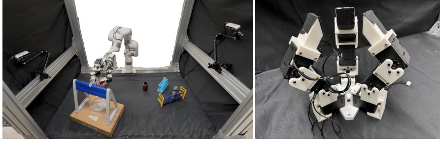
Figure 7: Three-finger Hand Used for the Liquid Handling Task. Left: The three-finger hand is approaching the pipette. Right: The three-finger hand consists of 9 degrees of freedom and uses a flat surface at the fingertips for better gripping performance.
