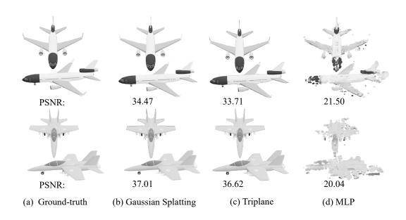
Figure 11: Ablations on 3D representation implementations. (a) The input shapes from ShapeNet. (b) Gaussians trained on the ground truth shape. (c) Reconstructed Gaussian primitives obtained with our Triplane-based Gaussian Variational Auto-encoder using proposed Gaussian Splatting functions. (d) Replace the Triplane architectures with simple MLPs.
