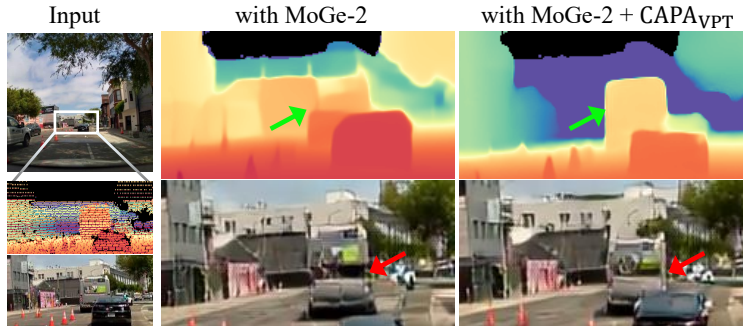
Figure S2: Novel view synthesis results using Gen3C, with depth map from Moge-2 and CAPA VPT . The viewpoint is moved by 1m higher than the input.
