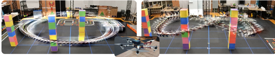
Figure 1: With only three minutes of manually collected data, the proposed algorithms for training neural stochastic differential equations yield accurate models of hexacopter dynamics. When used for model-based control, they result in policies that track aggressive trajectories that push the hexacopter’s velocity and Euler angles to nearly double their maximum values in the training dataset. Videos of experiments are available at https://tinyurl.com/29xr5vya .
