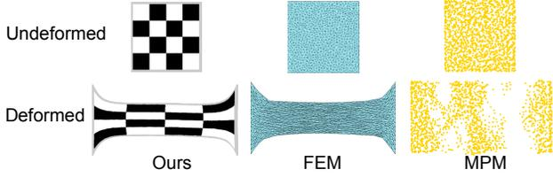
Figure 5. **Elastic tension test.** We use  $\alpha = 3$  hidden layers of width  $\beta = 68$  for our MLP, which takes the same memory as the FEM mesh (0.8K vertices, 1.5K faces) and MPM point cloud (1.7K points).
