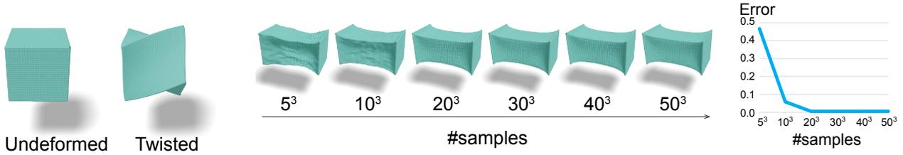
Figure 11. **Twisting test.** Quasi-static simulation in 3D. The right end is twisted 45 degrees.
