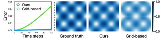
**Figure 3. 2D Taylor-Green vortex simulation.** Left: the mean squared error of the velocity field for 100 timesteps. Error is computed using  $48^2$  uniform spatial points. Right: velocity magnitude of solutions from the ground truth, ours, and the grid-based method (grid size 48) at timestep  $n = 100$ . Under the same memory usage (for storing the spatial representation), our solution has a significantly smaller error than the grid-based method.
