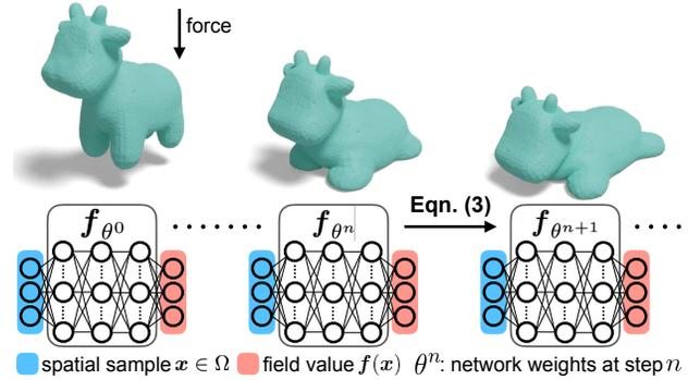
**Figure 1. Evolve neural field over time.** We represent the field of interest using a neural network  $\mathbf{f}_{\theta^n}$ , whose weights  $\theta^n$  are updated at each time step via optimization-based time integration (Equation (3)). In this case, the spatial domain  $\Omega$  is the volume encompassed by the undeformed object, and the represented field  $\mathbf{f}$  is the deformation map. The governing PDE is the elastodynamic equation.
