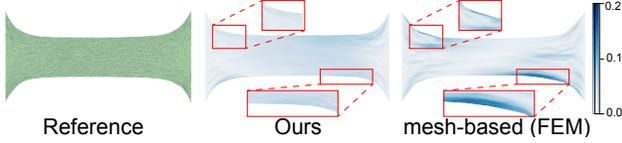
Figure 6. **Error of the elastic tension test.** We visualize the L2 distance error of our result and the FEM result (0.8K vertices). Errors are calculated against the reference result obtained by high-resolution FEM. Our result obtains smaller errors.
