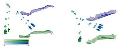
**Figure 11:** Spectral CoSMA embeddings of the YARIS front beams for 10 simulations, which deform in two branches. Color encodes timestep and branch.
