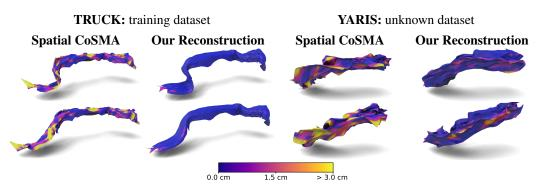
**Figure 5:** Reconstructed front beams from the TRUCK (length of 150 cm) at time t = 24 (test sample) from two crash simulations representing different deformation behavior and from the YARIS (length of 65 cm) at t = 15. The average Euclidean P2S error (in cm) of the faces is highlighted.
