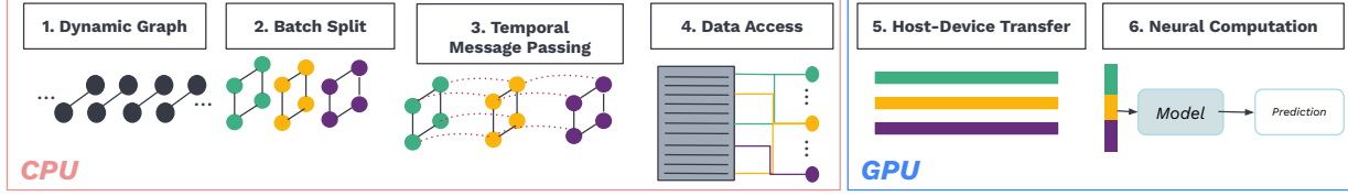
Figure 1. High-level data flow of temporal graph training. The input edge stream is first split into batches. Next, temporal neighbourhoods are computed, and feature data for the relevant nodes is read from storage. Features are moved to the GPU and forwarded to a model for computation.
