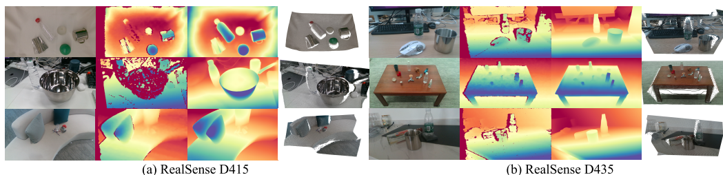
Figure 1: Generalizability of D 3 RoMa in the real world. Our method robustly predicts transparent (bottles) and specular (basin and cups) object depths in tabletop environments and beyond. RGB image, pseudo colored raw disparity map, our prediction, and point cloud are displayed for each case of a total of 6 frames captured by camera RealSense D415 and D435. * RGB and depth images are not aligned for the D435 camera for better visualization.
