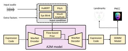
Figure 8: The network structure of A2M model. Dotted lines denote the processes that are only executed during the training phase in Sec. 3.4.
