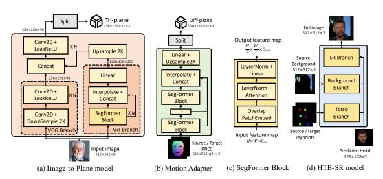
Figure 2: The network structure of I2P model, motion adapter, and HTB-SR model.
