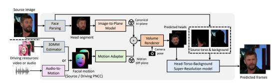
Figure 1: The inference pipeline of Real3D-Portrait. With one source image as input and a video/audio as driving condition, it synthesizes 3D talking avatars with a realistic torso and background.
