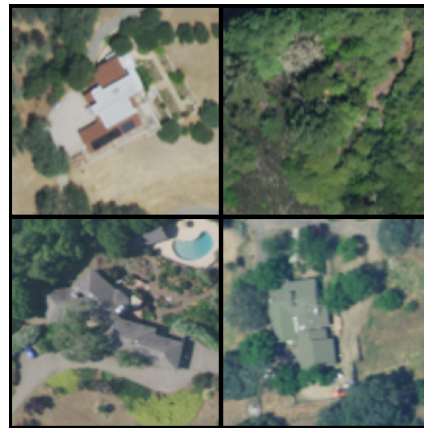
Figure 1: Sample of NAIP Labels: These are four examples of our NAIP samples. The two houses on the first column were destroyed, whereas the ones in the second column survived the fire. Notice the image in the right-upper corner represents some of the labeling issues in our database, we remove all image labels where more than 95% of pixels are vegetation (using the NVDI).
