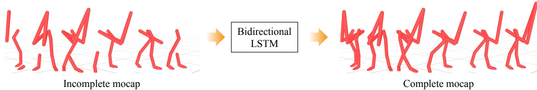
Figure 5: Visualization of the mocap prediction process. Left: the original incomplete data. Right: the complete data after predicting the missing markers with a bidirectional LSTM. Segments are drawn between pairs of existing markers.
