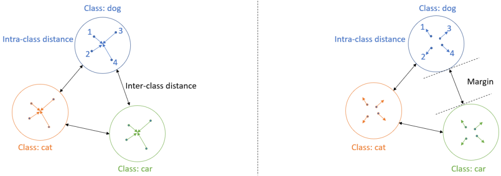
Figure 1: In most distillation methods, the teacher model is trained such that samples from different classes are separated from each other while samples from the same class are brought closer together, as illustrated in the left. However, as the intra-class distance decreases, the intra-class information within the soft labels may be lost. The proposed intra-class contrastive loss encourages an appropriate increase in intra-class distance. We also introduce a margin to ensure the stability of inter-class distances, as shown on the right.
