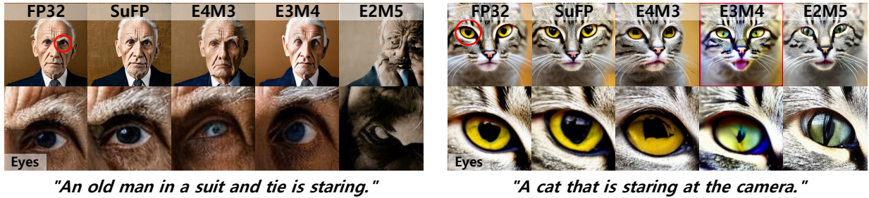
Figure 6: (a) Comparison of sample images and (b) details of images generated by the Stable Diffusion model on the COCO dataset using FP32, SuFP, and FP8 representations (E4M3, E3M4, and E2M5). Note that E5M2 is excluded from the comparison because it fails to generate images. SuFP follows the original FP32 images more closely than other FP8 representations, which indicates accurate quantization.
