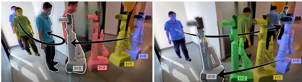
Figure 1: Left: Standard MPC efficiently cuts blind corners, forcing the human to back up; Right: Social Performer-MPC avoids cutting blind corners, enabling safe navigation around humans.
