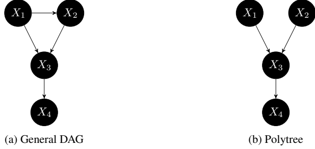
Figure 2: (a) A general DAG may contain undirected cycles, as between X_1 - X_2 - X_3 - X_1 . (b) A polytree cannot contain undirected cycles so could not have an edge between X_1 and X_2 without first removing another.
