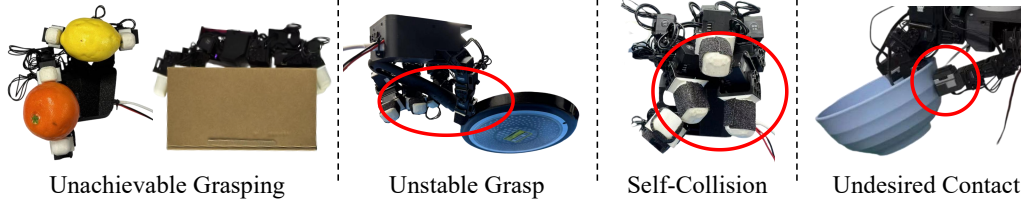
Figure 2: The challenges of previous retargeting-based dexterous teleoperation systems. Unachievable Grasping shows poses that are physically infeasible for human hands. Unstable Grasp leads to object dropping due to weak contact. Self-Collision indicates finger interference during motion. Undesired Contact refers to insufficient contact between the tactile sensor surfaces and the object.
