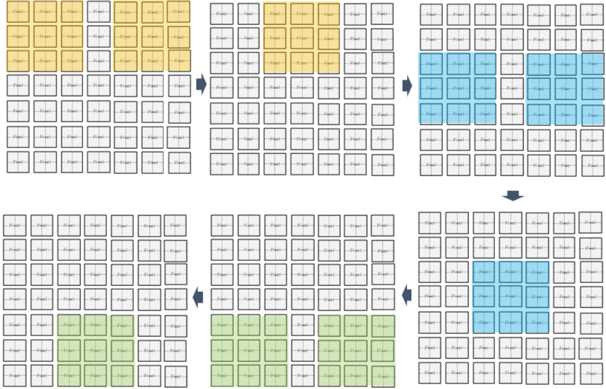
Figure 4: The schematic diagram of the convolution process.
