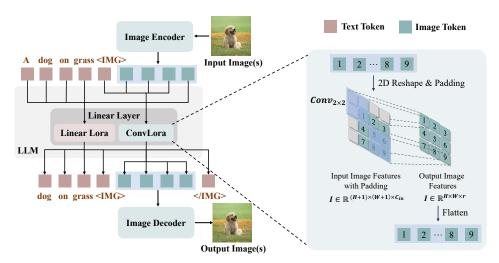
Figure 2: An autoregressive VLG with our proposed MoSS added to its linear layers. The linear LoRA on the left side is specialized to generate text tokens and the Convolutional LoRA on the right side is specialized to generate image patches. On the right handside, we show the details of convolutional operation applied to autoregressively generate image tokens. Best viewed in color.
