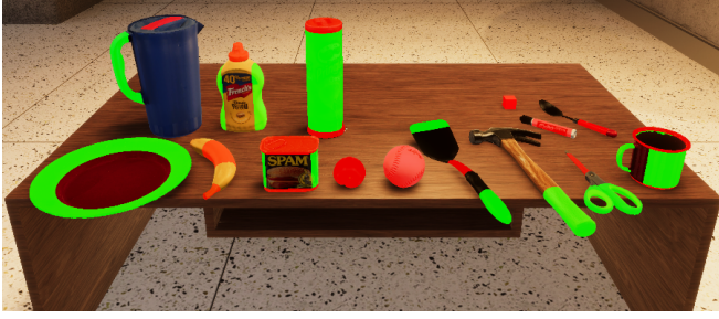
Fig. 3: The 15 YCB objects with labeled object parts. The red and green masks encode the top and side grasps , respectively. The non-highlighted object parts are labeled as no grasp .
