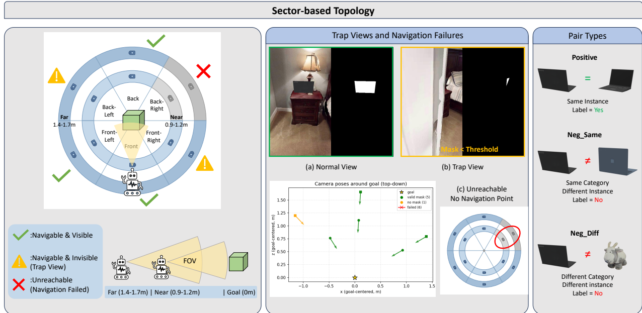
Figure 2. Sector-based navigation topology and protocol-level annotations. Left: 6 active sectors spaced every 60^\circ at two observation distances (far: 1.4–1.7 m; near: 0.9–1.2 m). Each sector is navigable & visible (✓), a trap view (△, navigable but mask below threshold), or unreachable (✗, no navigable point). Center: Examples of a normal view, a trap view, and an unreachable sector with corresponding top-down camera poses. Right: Three pair types used in evaluation: positive (same instance), neg_same (same category, different instance), neg_diff (different category).
