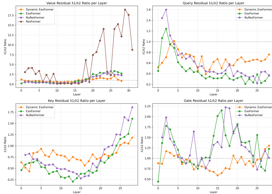
Figure 4: The ratio \lambda_{n,1}/\lambda_{n,2} plotted for each component ( Q, K, V, G ) across layers for models using elementwise mixing for model variants \sim 450M . Values greater than 1 indicate stronger reliance on the anchor signal, while values less than 1 indicate preference for current-layer projections.
