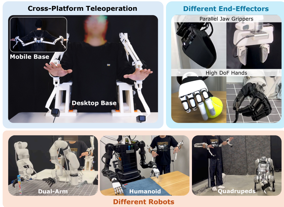
Figure 1: An Overview of the Proposed ACE System. The system consists of two bimanual exoskeleton arms and two cameras for hand pose tracking. Together with our modular design of the base, we can perform teleoperation across a wide range of end effectors and robot platforms.
