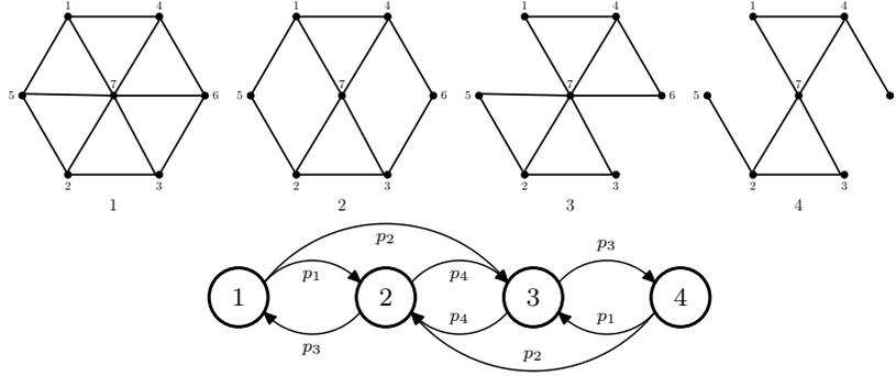
**Figure 1:** [Top] Hexagon topologies arranged in a Markov chain with four states. [Bottom] The state transition diagram for the four states.
